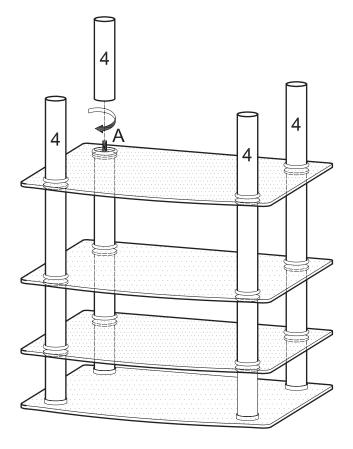
Screw cylinders (4) onto long rods (A). Note that cylinders (4) will fit snuggly inside the decorative rings placed in the previous step.
